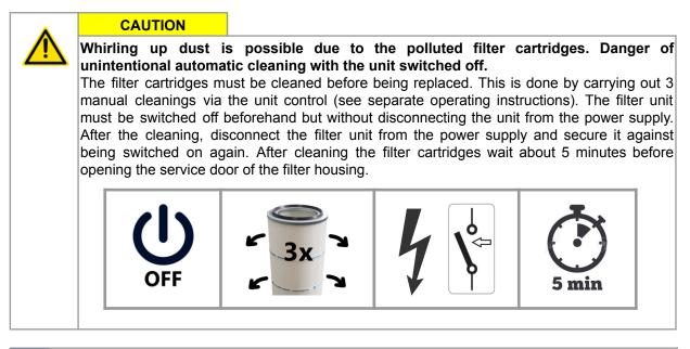
We recommend using a disposable protective suit when changing the filter cartridges.
