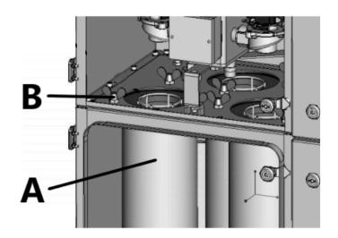
Before changing the filter cartridges hold ready an appropriate container (e.g. PE bag) for disposal.
